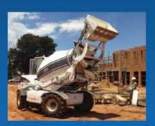
Easy-to-Manoeuvre Four Wheel Drive True Batching Plant
