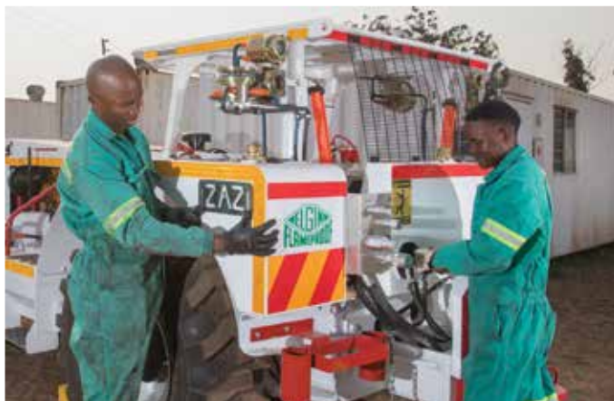
Izazi's new Elgin 4x4 underground flameproof tractor being prepared for transport to site.
