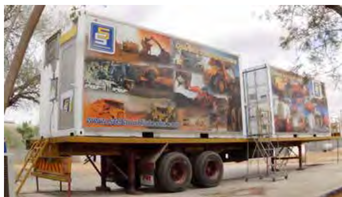
One of the mobile operator training simulators, including a classroom, that can accommodate up to six learners, on the right, and the simulator room that accommodates the console and three-dimensional simulation software and screens, on the left.
