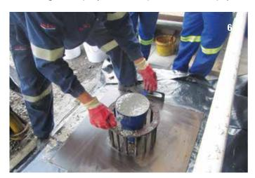
rated as a quality level 2 for Eskom. In order to ensure compliance with this quality level, the cementitious grout proposed by Stefanutti Stocks was sent to an approved laboratory where it was tested for compressive strength, tensile strength, shrinkage cracking, durability index, oxygen permeability index, water absorptivity index and tensile pull-off bond strength.
