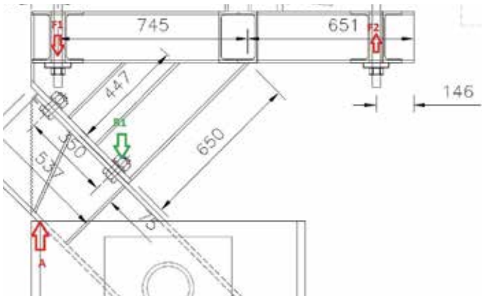
For the casting case the force at F1 is downwards and the force F2 is upwards resulting in a tension force at R1 with a magnitude of 655 kN.
